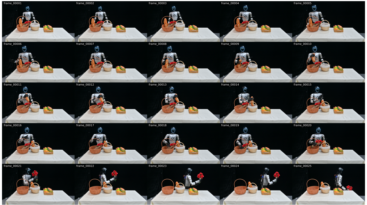
Figure 9: Complete snapshot of Obstacle-Avoidance Basket Carrying.
